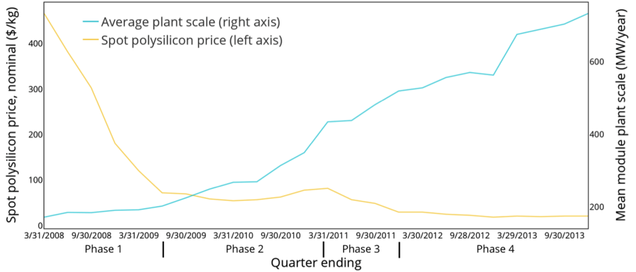
Figure 4: Between 2008 and 2013, the average size of module manufacturing facilities increased and the price of polysilicon decreased.
